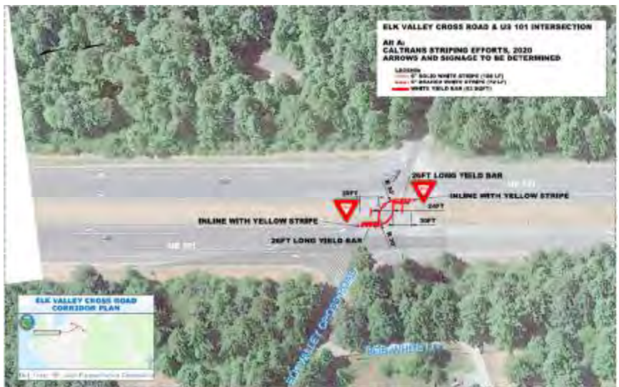
Figure 4: EVCR/US 101 Intersection Striping
